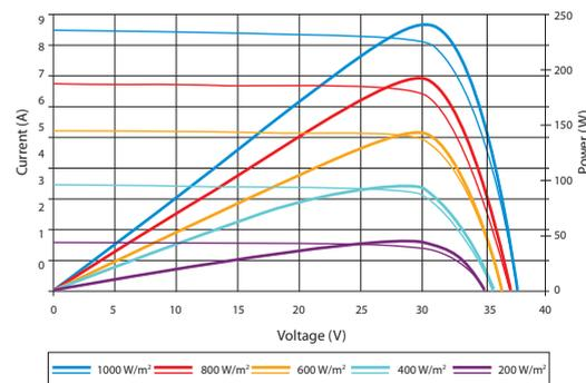
Excellent performance under weak light conditions: at an irradiance intensity of 200 W/m<sup>2</sup> (AM 1.5, 25 °C), 95.5% or higher of the STC efficiency (1000 W/m<sup>2</sup>) is achieved
